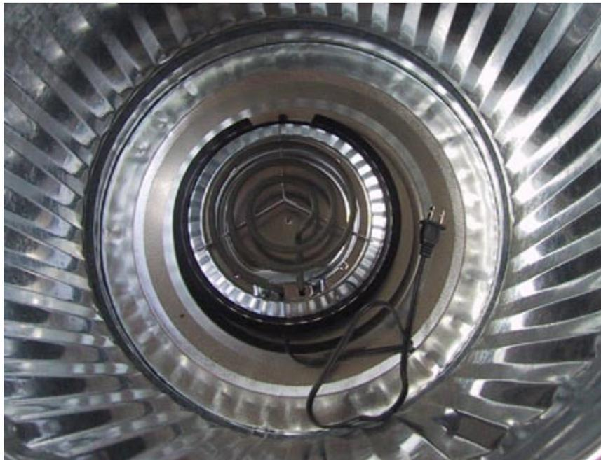
So the plan is simple, use an electric hot plate to heat wood chips inside a metal trash can.
