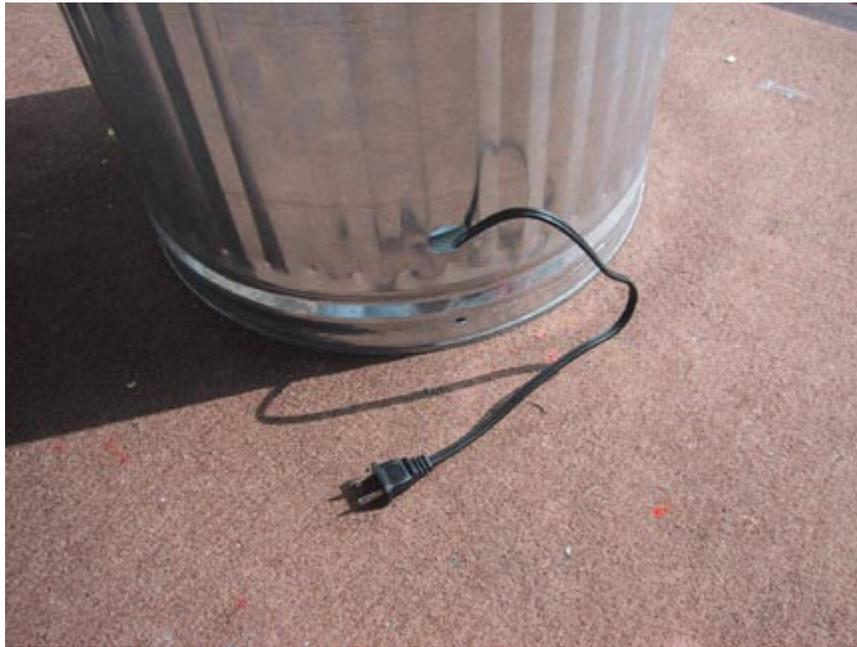
I used a drill and metal nibbler to open a hole in the trash can. Be sure to file down the edges so that the power cord can't get cut.
